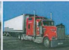
Class 8 Kenworth W900 tractor with spread-axle 48 feet (15 m) refrigerated trailer.
