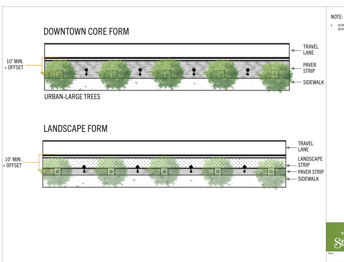
SETBACK DISTANCE MAY INCREASE PER ROAD SPEED LIMIT, SEE SHEET A-1 FOR MORE DETAILS. SETBACK DISTANCES ARE MEASURED FROM THE EDGE OF TRAVEL WAY TO THE CENTER OF TREE TRUNK.
