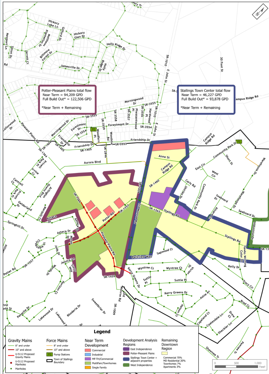
Existing Sanitary Sewer in Town of Stallings West Sanitary Sewer at Full Build-Out
