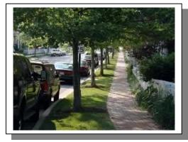
benefit. Planting strips should not be less than 4-feet in width. The recommended planting width to permit healthy tree growth is 6 to 8 feet measured from the edge of pavement or back of curb. While planting strips are the preferred means of providing a buffer, they are not always feasible or appropriate. Areas of high foot traffic may preclude landscaping due to maintenance or space considerations. Additional information about street trees is provided on the following page.
