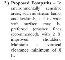
All trails should be maintained with a 5 ft. cleared area from the edge of the trail on each side. Pitch trails to drain with a 2% minimum grade. Paving materials may vary in specific locations.
