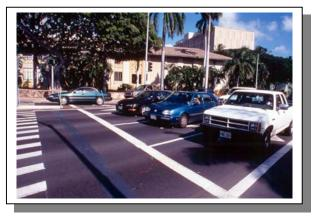
cannot be located exactly where vehicles are expected to stop, the stop bar should be placed at the desired stopping point. Finally, the stop bar should be placed so that vehicles have optimum sight distance along the intersecting roadway."
