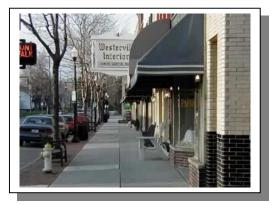
streetlights, street signs, fire hydrants, parking meters, etc., are placed in the buffer zones so as not to restrict pedestrian flow in the travel path. The buffer zone may be a good location to use paver stones for easy and affordable access to underground utilities.
